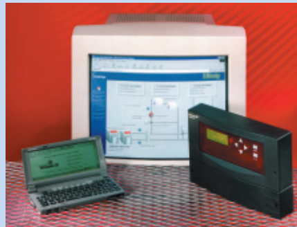
A BEMS provides vital, up-to-date information for the control of plant
